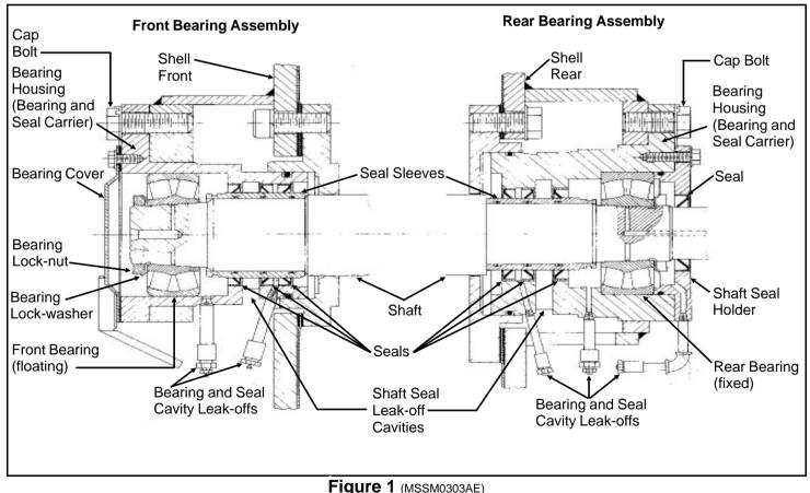
Cross Section View of Front and Rear Bearing Assemblies (Bearing Assembly for 60" and 72" WED Shown. Others similar.)
