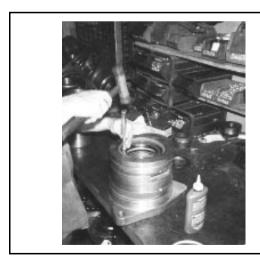
FIGURE 5 (MSSM0303AE) Installing Seals in Bearing Housing
